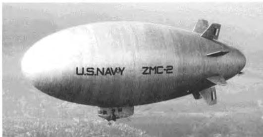
The ZMC-2, shown here on a flight over Washington, D.C., was the only metal-clad airship. It was scrapped in 1941 after 12 years in service. It would have put up quite a radar signature, eh!
