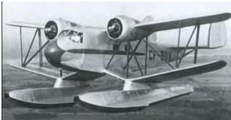
The Canadian Fleet 50 design began in 1936 and the first flight was in 1938. The design included several innovative construction techniques. Because it was underpowered only five were built.
