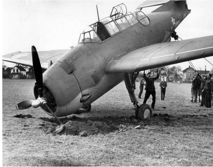
The origin of this TBF (TBM?) photo is unknown but there's some interesting observations (other than the parking technique): No carrier hook, Wing and Horizontal stabilizer leading edge cover, little if any identification markings other than the US Marine Insignia Star with the Red Dot - which was not used after May 1942. This leads your editor to wonder if this was a Marine training aircraft (note rear cockpit canopy open) for land operations only?
