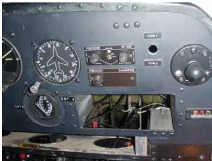
Removed Radio Holes
