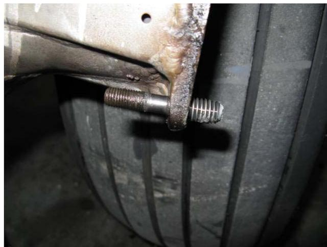
Note the pulled out exhaust stud still in the exhaust manifold after it was removed and set against a main wheel tire. Aside from low compression, one of the removed cylinders had two exhaust studs that were loose in the cylinder heads.
