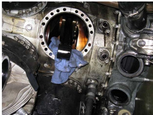
This is the area where the number 11 cylinder sat before being removed. MANY parts had to come off before we were able to remove the cylinder itself.
